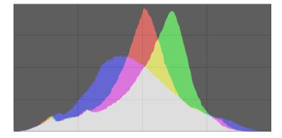
The histogram shows the distribution of pixels by lightness for each color channel.
