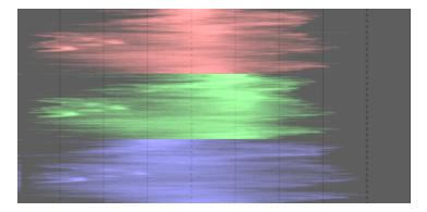
The RGB parade can be useful for matching the intensities of the red, green, and blue channels. It can also help to understand the differences between, and individual qualities of, each channel.
