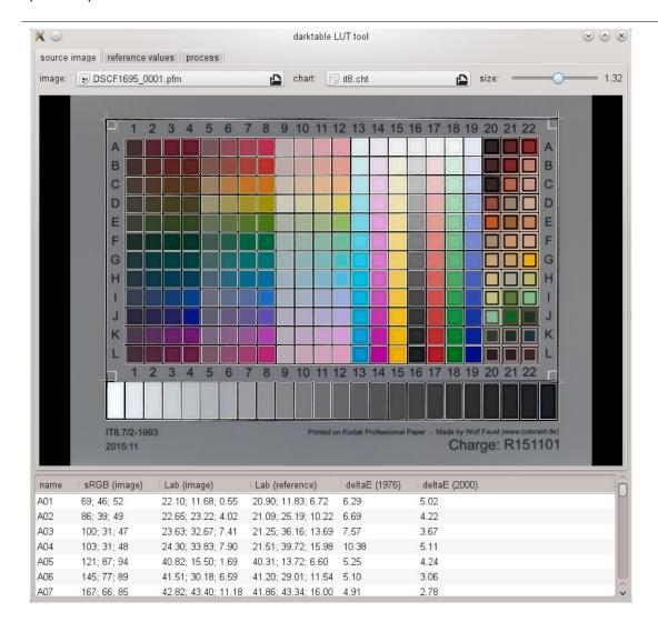
In real life the photo taken from the color reference card will show some perspective distortions relative to the layout defined in the chart file. For that reason the layout is displayed as a grid over the image and can be modified.
