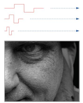
These wavelet functions are used to scan and decompose an image using a mathematical operation called convolution. This picks out details from the image that are on a similar scale to the size of a given wavelet, and builds a number of these detail layers, each corresponding to a different wavelet scale.
