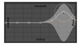
Here, each node in the graph represents a different level of detail in the image, from coarse detail on the left to fine detail on the right. You can raise or lower each of these nodes with your mouse to increase or decrease the module's effect, respectively, on that wavelet scale.
