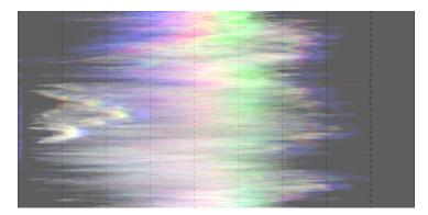
In the vertical waveform, the vertical axis of the plot represents the vertical axis of the image, and the horizontal axis represents the distribution of pixels by lightness. The vertical waveform can be useful for portrait-format images, or simply to understand an image in a different way.
