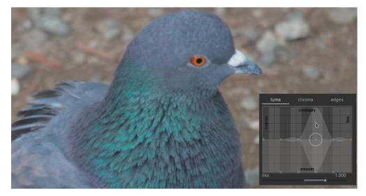
Raising the two control points at the right-hand end of the graph will increase the sharpness of the fine details (the eye and feathers of the bird) while leaving coarser details (the rocks in the background) largely unaffected. The example below has been exaggerated to better illustrate the effect.
