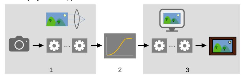
1. Scene-referred modules process linear data that is proportional to the amount of light collected by the camera at the scene. The dynamic range of an image in the scene-referred section of the pixelpipe is often larger than that of the display medium.
