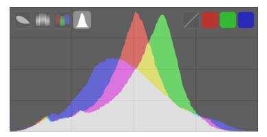
Hover the mouse over the module to reveal buttons that can be used to adjust the display. The buttons on the left-hand-side are used to choose the display mode, from left-to-right: vectorscope, waveform, rgb parade and histogram. The buttons on the right-hand-side control how the plot for the current scope is drawn.
